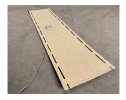
The Shoot is a patented insulation backer used as a substrate for spray foam and blown insulation in open framed areas of new construction applications for residential and commercial buildings. Pre-creased staple flanges allow for easy installation in most common wall cavities. The Shoot is ideal for knee walls, common walls and any open cavity without a spray template.
